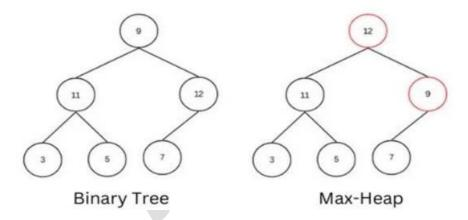
After swapping the root node with the last element in the heap, the visualized heap will now have one less element.
