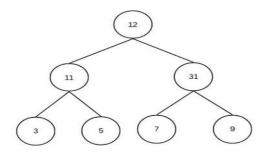
3. Convert the Binary Tree Into a Max Heap: all parent nodes must have values that are greater than or equal to the values of their children. this means swapping node 12 and node 31 positions in the tree to satisfy the requirements for a max-heap tree
